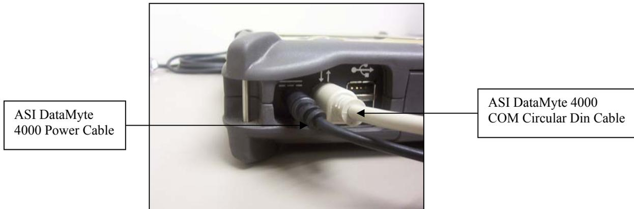
FIGURE 2.1 D - Bottom View of ASI DataMyte 4000 (Power / Serial Communication to PC).
