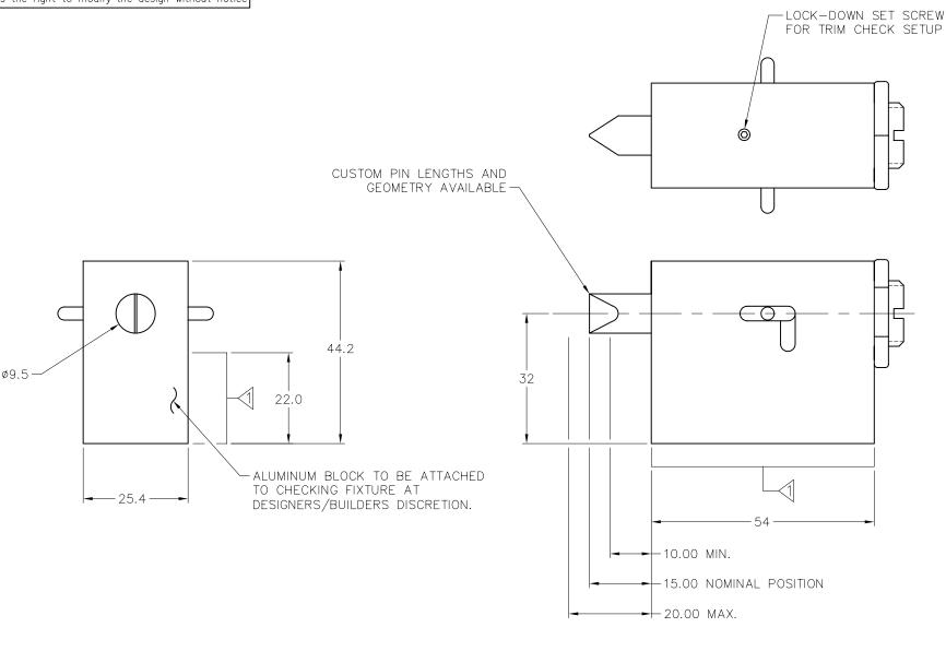
BRACKET SHOWS ALLOWABLE AREA FOR BOLT HOLE PATTERN AND DOWELING.
