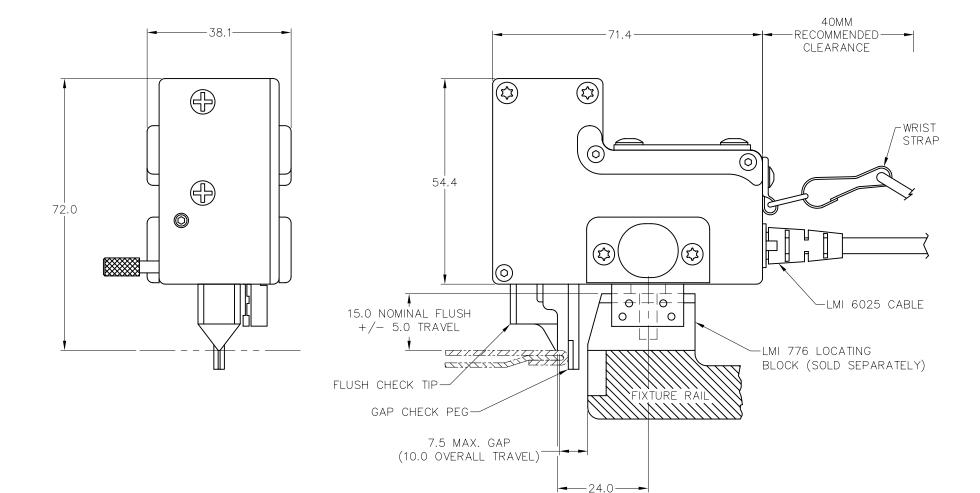
NOTE: 10MM OF TRAVEL FOR BOTH FLUSH AND GAP CHECKS.
