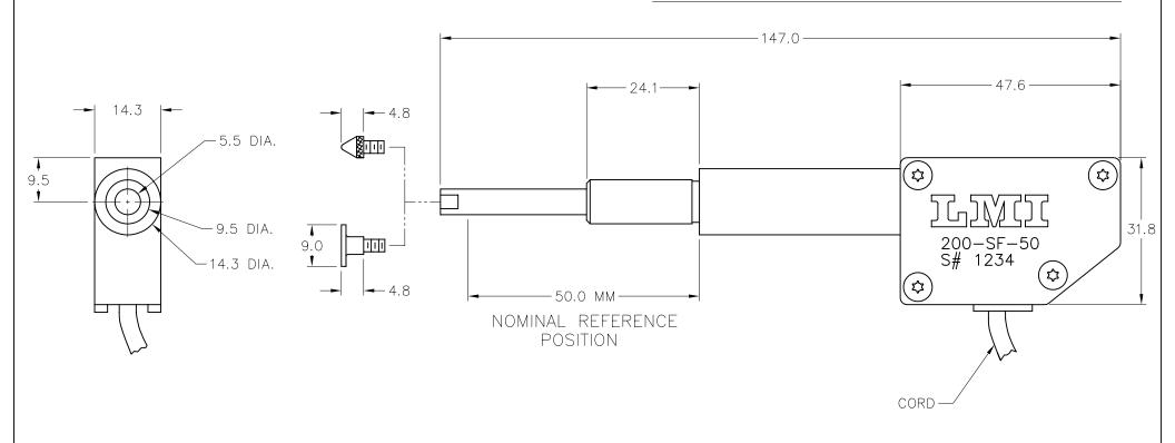
9.5 DIA. SHAFT ON TRANSDUCER TO FIT LMI261 ADJUSTABLE THREADED BUSHING OR STANDARD 3/8" DIA. BUSHING
