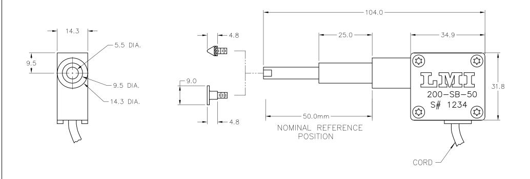
9.5 DIA. SHAFT ON TRANSDUCER TO FIT LMI261 ADJUSTABLE THREADED BUSHING OR STANDARD 3/8" DIA. BUSHING
