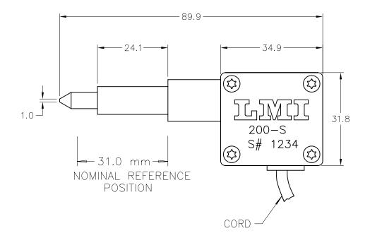
9.5 DIA. SHAFT ON TRANSDUCER TO FIT LMI261 ADJUSTABLE THREADED BUSHING OR STANDARD 3/8" DIA. BUSHING
