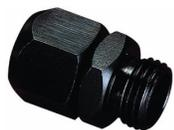
Insert the LMI 5200 probe into the collet and align the retracted tip with the outside edge of the holding block. Hand-tighten the collet using the hexagonal nut. The internal fingers of the collet will grip the barrel of the probe with equal and dispersed pressure preventing the probe from sliding closer to or further away from the part to be measured.
