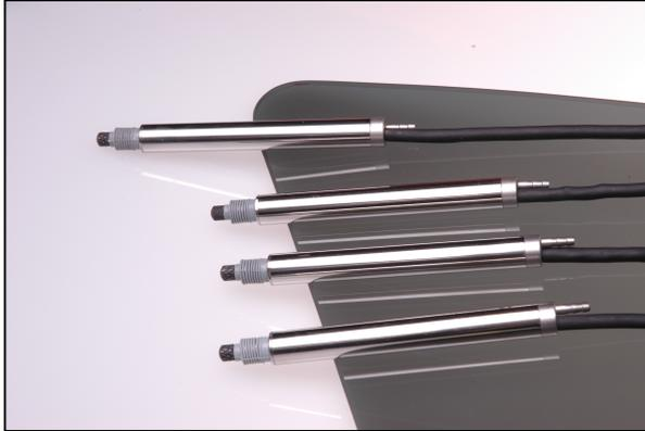
LMI 5300 probes extend to meet the part when air is supplied to the probe. Each probe has a 10mm range of travel with an accuracy of +/- .03 mm. Each probe has five main components:
