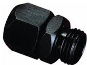
Insert the LMI 5300 probe into the collet and align the retracted tip with the outside edge of the holding block. Hand-tighten the collet using the hexagonal nut. The internal fingers of the collet will grip the barrel of the probe with equal and dispersed pressure, preventing the probe from sliding closer to or further away from the part to be measured.
