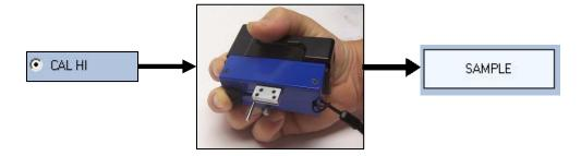
3. If the Low and High calibration is good, the software will automatically advance to the CAL Master position. Fully insert the 241W into the master block and click the SAMPLE button.
